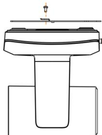
5. Push forward camera's bottom slide according to the mounting plate's bottom slide until they reach their limit. Fix the ceiling mount plate and camera's bottom plate with M3x8 screws.
