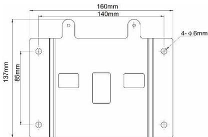
2. Fix the mounting plate onto the ceiling or cement roof with 4 screws which should be prepared by you.
