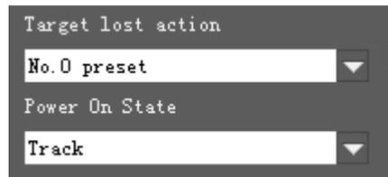
**Target Lost Action:** Used to define the action to be performed if the camera loses the tracked object for a period of time.
