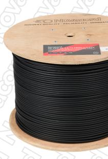
High-frequency coaxial cable, for low-loss RF radio communication systems. Coaxial cable used in cable broadBand communication networks designed according the European Standard EN 50290-2-20. Operating at frequencies between 5 MHz and 10000 Mhz. Cable designed to avoid the release of toxic matter in case of fire because they do not contain any halogens.
