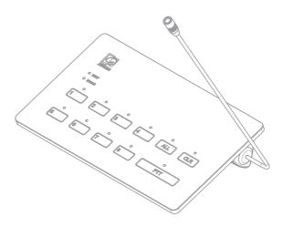
The front panel of the MPX contains various selectors and indicators. All selection buttons are implemented using capacitive touch principle, whereby selection is done by gliding your finger over it.
