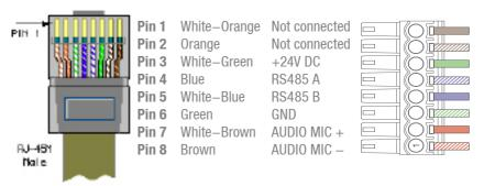
The microphone should be connected to the matrix system using the fixed connection cable with a length of 2 meters. The distance can be extended to a maximum length of 300 meters, using CAT5E (or better) twisted pair cabling.
